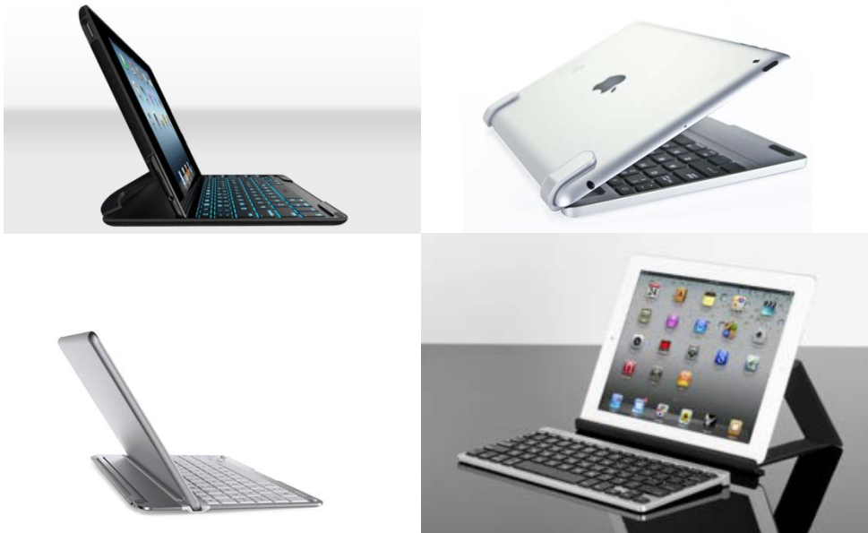
Figure 4. Different types of external keyboards for tablets. Folio case, upper right; Clamshell, upper left, keyboard shell, lower right, stand-alone keyboard, lower right
